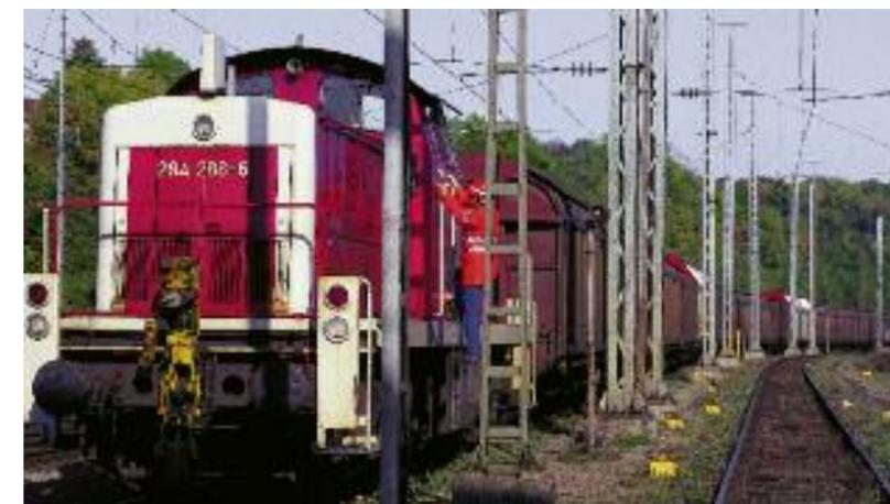
MTU tested out an exhaust recirculation system for 5,000 hours under everyday working conditions on a V297 Class shunter.
